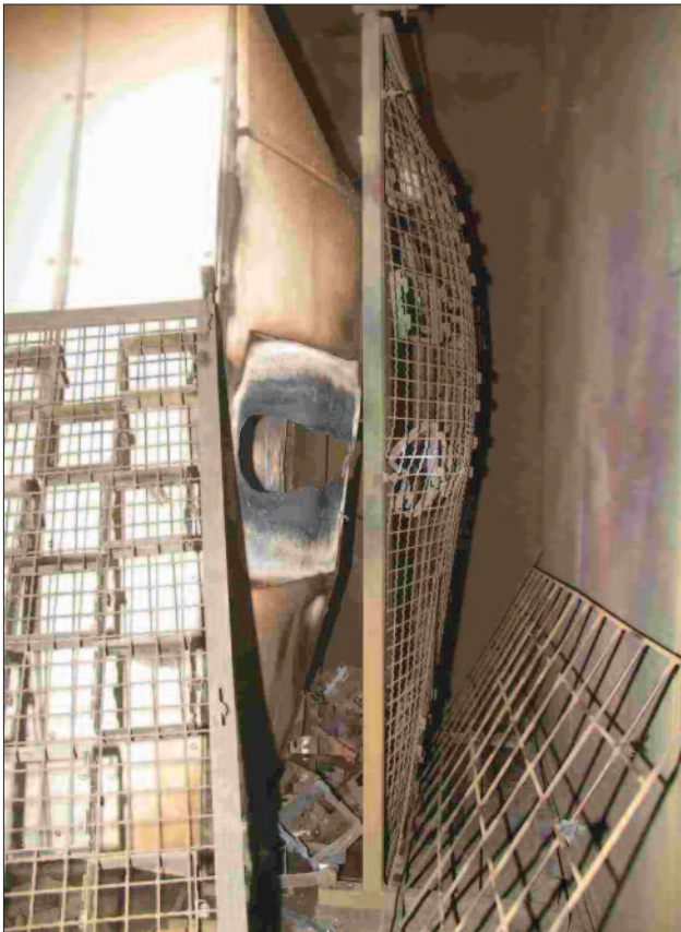
Early stage testing to ensure final design achieves all 5 criteria of Annex A IEC 62271-200
