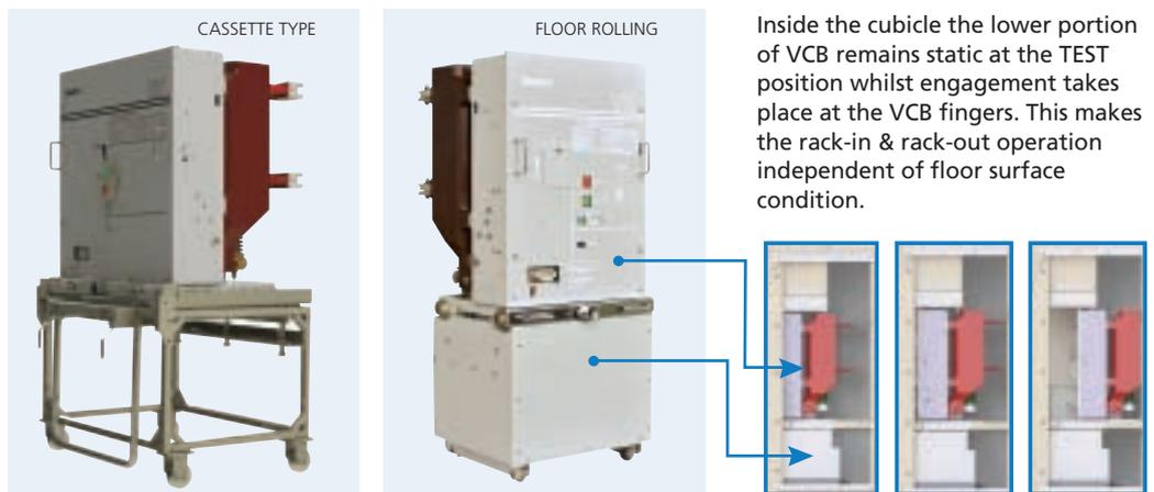
Inside the cubicle the lower portion of VCB remains static at the TEST position whilst engagement takes place at the VCB fingers. This makes the rack-in & rack-out operation independent of floor surface condition.
