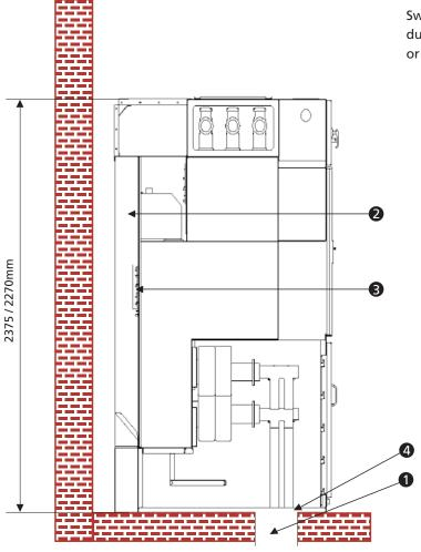
Switchgear installation with rear pressure relief duct (option) for switchgear blocks with IAC A FL or FLR up to 31.5kA/1s
